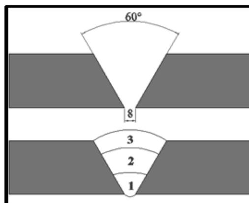
**Figure 1. Scheme of joint preparation of FCAW weld, V shaped groove design and number of welding passes**
