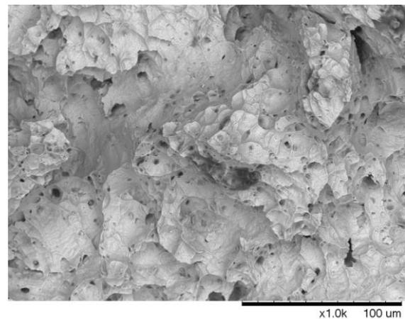
Figure 8. Fracture morphology of SEM images of the samples welded under 100%CO<sub>2</sub> shielding gas
