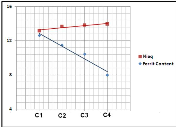
Figure 4. The affection of CO<sub>2</sub> in the gas composition on Nieq ve delta-ferrite values
