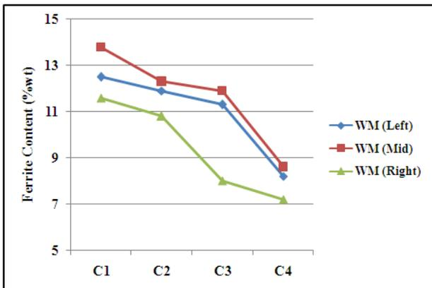
Figure 5. Variation of % wt content of ferrite in the weld metal
