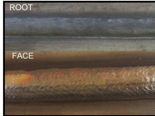
Figure 3. Appearance of the weldment by FCAW methods
