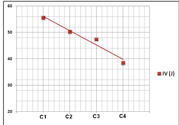
Figure 7. Variation of the notch impact energy values depending on CO<sub>2</sub> content in the shielding gas
