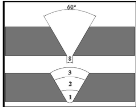
**Figure 1. Scheme of joint preparation of FCAW weld, V shaped groove design and number of welding passes**
