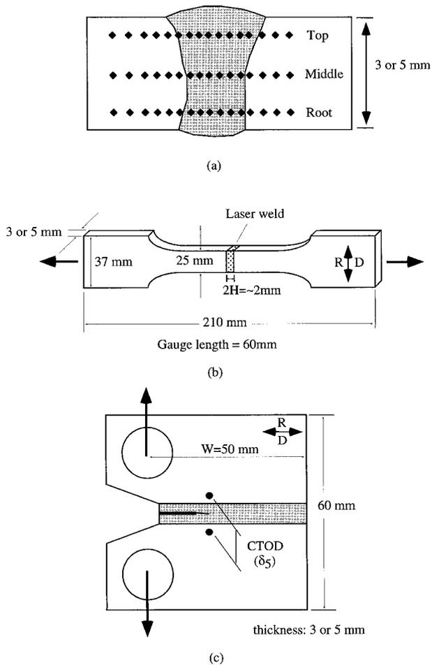
*a* hardness measurements; *b* tensile test specimen; *c* compact tension (CT) specimen with local crack tip opening displacement (CTOD) measurement technique of  $\delta_s$
