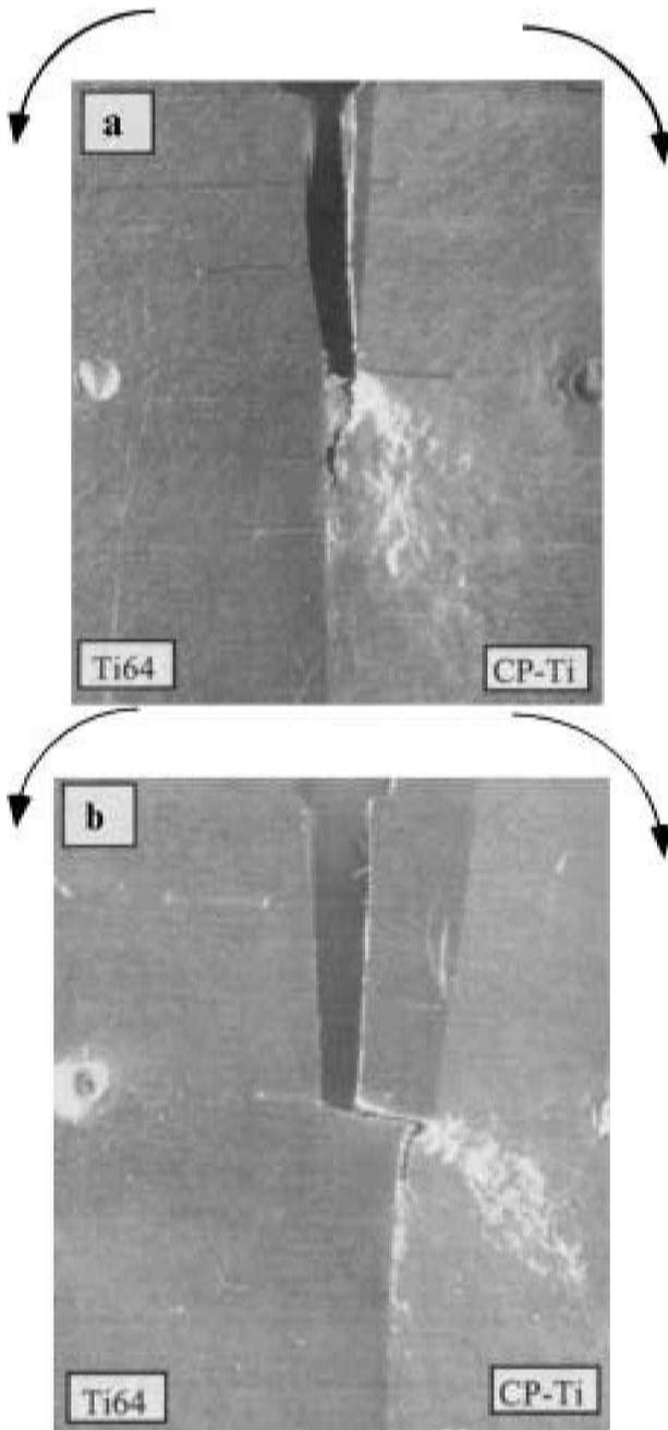
a interfacial crack specimen, in which ductile crack growth occurs within CP Ti adjacent to interface; b subinterfacial crack specimen, in which crack grows perpendicular to interface and deviates into lower strength CP Ti, with subsequent ductile fracture within CP Ti adjacent to interface
