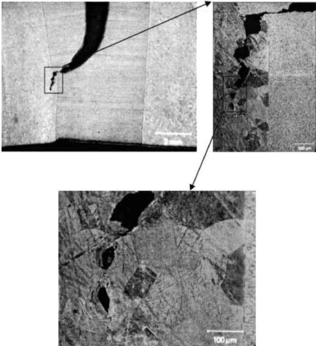
**15 Crack path deviation into lower strength side block (CP Ti) and crack growth involving void formation and coalescence within side block adjacent to interface in strength overmatched strong bond specimen with interlayer thickness of 5 mm (optical)**
