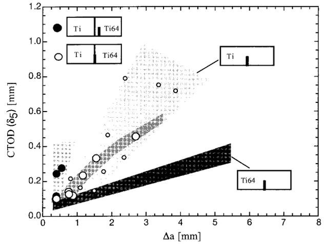
7 Comparison between R curves (CTOD  $\delta_5$  versus increase in crack length  $\Delta a$ ) for base materials and dissimilar joints
