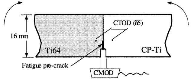
**2 Schematic illustration of crack tip opening displacement (CTOD  $\delta_5$ ) measurement during four point bend tests using clip on gauge with 5 mm gauge length over fatigue crack tip**
