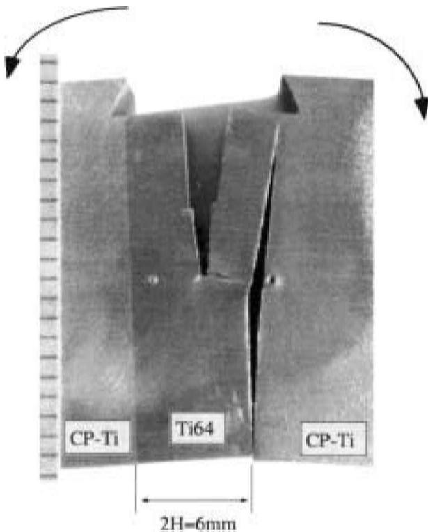
**10 Crack deviation from stronger Ti64 interlayer into softer CP Ti side block and brittle debonding along interface due to weak bonding in strength over-matched weak bond specimen with interlayer thickness 2H=6 mm (optical)**
