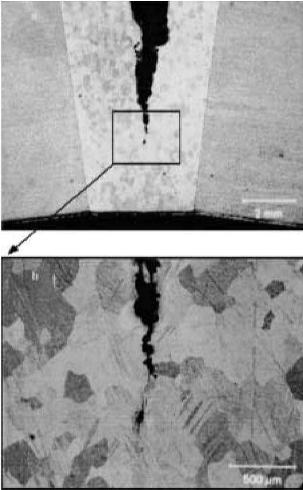
**13 Crack growth involving void formation and coalescence in softer interlayer of strength undermatched strong bond specimen with interlayer thickness of 5 mm (optical)**
