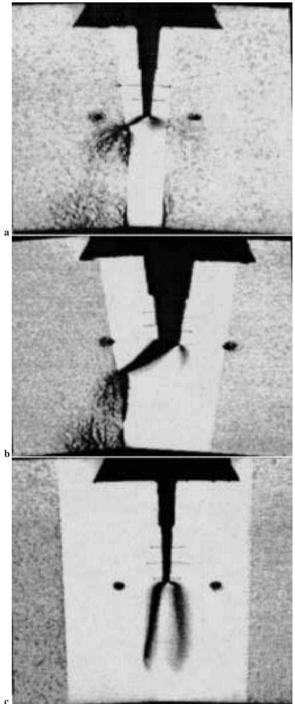
**14 Crack growth in strength overmatched strong bond specimens with interlayers of thickness a  $2H=2$  mm, b  $2H=5$  mm, and c  $2H=10$  mm (optical)**
