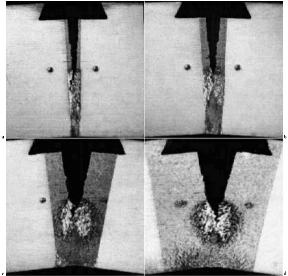
**12 Crack growth in strength undermatched strong bond specimens with interlayers of thickness *a*  $2H=1$  mm, *b*  $2H=2$  mm, *c*  $2H=5$  mm, and *d*  $2H=10$  mm (optical)**
