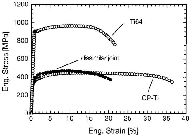
**4 Stress-strain curves for base materials and dissimilar joint used in present study**
