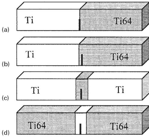
*a* dissimilar joint with interfacial crack; *b* dissimilar joint with subinterfacial crack; *c* strength overmatched joint; *d* strength undermatched joint
