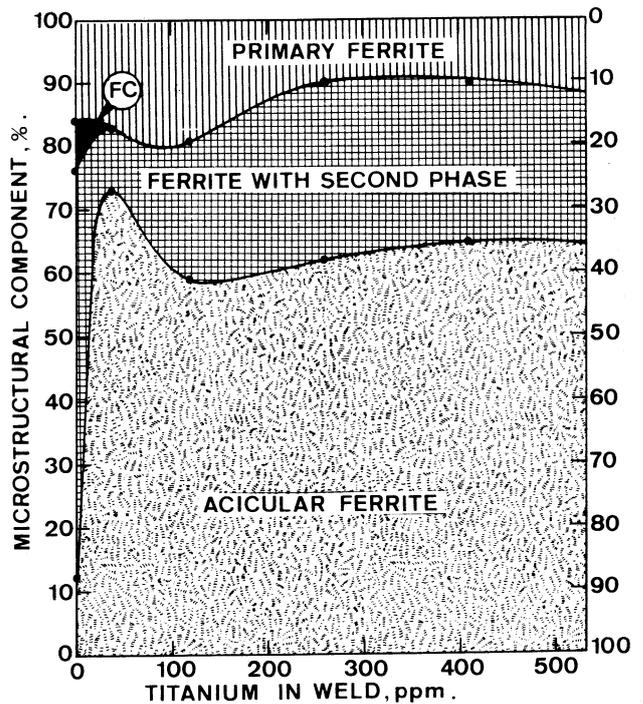
FIG. 2 EFFECT OF TITANIUM ON THE MICROSTRUCTURE OF AS-DEPOSITED WELD METAL
