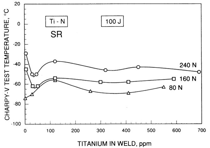
Fig. 8 EFFECT OF TITANIUM AND NITROGEN ON THE CHARPY-V TEMPERATURE CORRESPONDING TO 100 J
