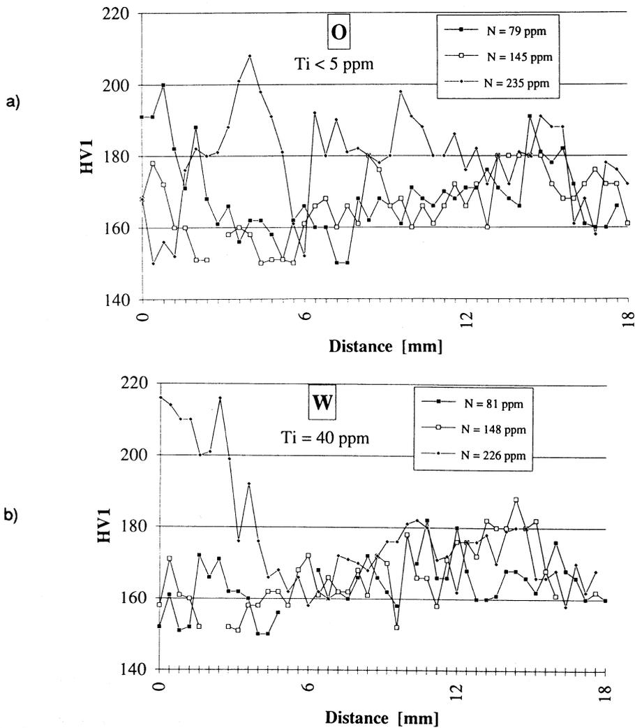
FIG. 7 HARDNESS TRANSVERSE RESULTS OF THE O, W, X WELD METALS FOR DIFFERENT NITROGEN CONTENTS
