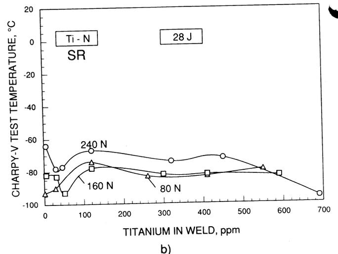
Fig. 9 EFFECT OF TITANIUM AND NITROGEN ON THE CHARPY-V TEMPERATURE CORRESPONDING TO 28 J
