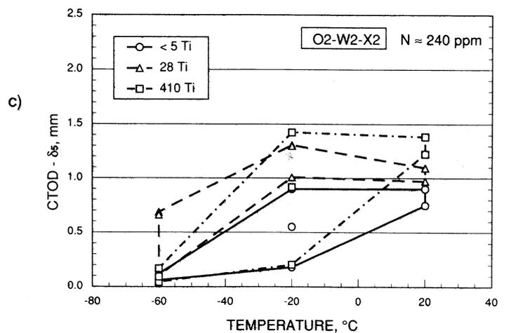
FIG. 10 EFFECT OF NITROGEN ON THE CTOD ( $\delta_s$ ) TOUGHNESS OF THE WELD METALS TESTED IN AS-WELDED CONDITION AT THREE TEST TEMPERATURES
