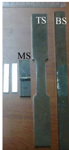
Figure 4 Metallographic (MS), tensile (TS), and bend (BS) test specimens extracted from the welded plates (see online version for colours)
