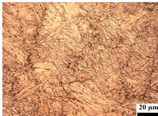
Figure 14 Microstructure of LTT 3 weld nugget (see online version for colours)
