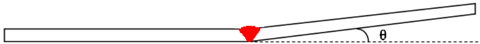
Figure 5 Measurement of angular distortion of the welded steel plates produced (see online version for colours)
