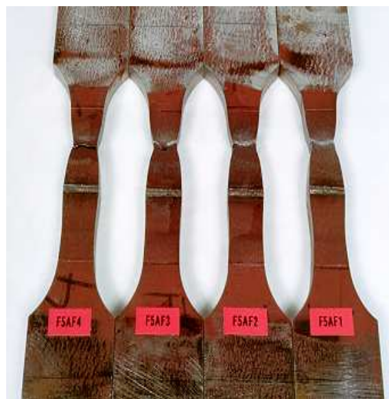
Figure 4. Typical strength overmatched flat tensile specimens failed away from the weld zone.
