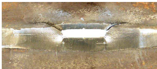
Figure 2. Fracture path deviation into lower strength base metal of the centre cracked wide plate under tension. The weld metal exhibits strength overmatching.
