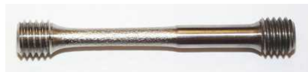
Figure 14. Post-test view of the bi-material round tensile specimen between ferritic and austenitic steels joined using diffusion bonding process.
