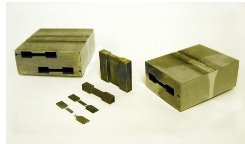
Figure 6. Extraction of micro flat tensile specimens from EB weld [10]
