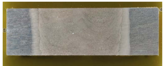
Figure 8. Macrograph of service exposed P22 butt joint – middle
