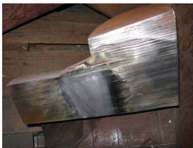
Figure 2. As-received nozzle sections (100 mm thickness welded to 150 mm thick material) after cutted into two pieces and etched for identification of weld area.
