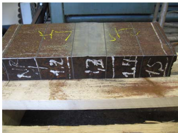
Figure 1 b. As-received outlet header used for the characterization of service exposed 145 mm thick base material with butt joint.
